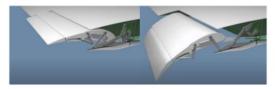
Combination of planar 4-bar mechanisms, actuated by one angular eletric motor
